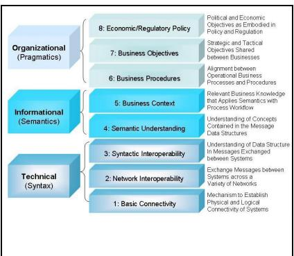
The GWAC Stack, a model created by the Gridwise Architecture Council, shows the many layers of interoperability.
